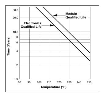
Figure 6-1. Qualified Life vs. Ambient Temperature.
